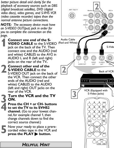
The S-VIDEO and VIDEO AV2 in(puts) are in parallel. The S-VIDEO input is dominant when in use. If separate video signals are connected to the S-VIDEO and VIDEO AV2 in(puts), the signal from the VIDEO AV2 in(puts) will not be usable.
